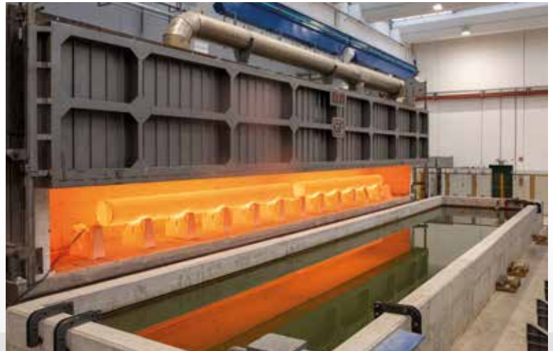
Fully automated loading and unloading heat treatment plant
