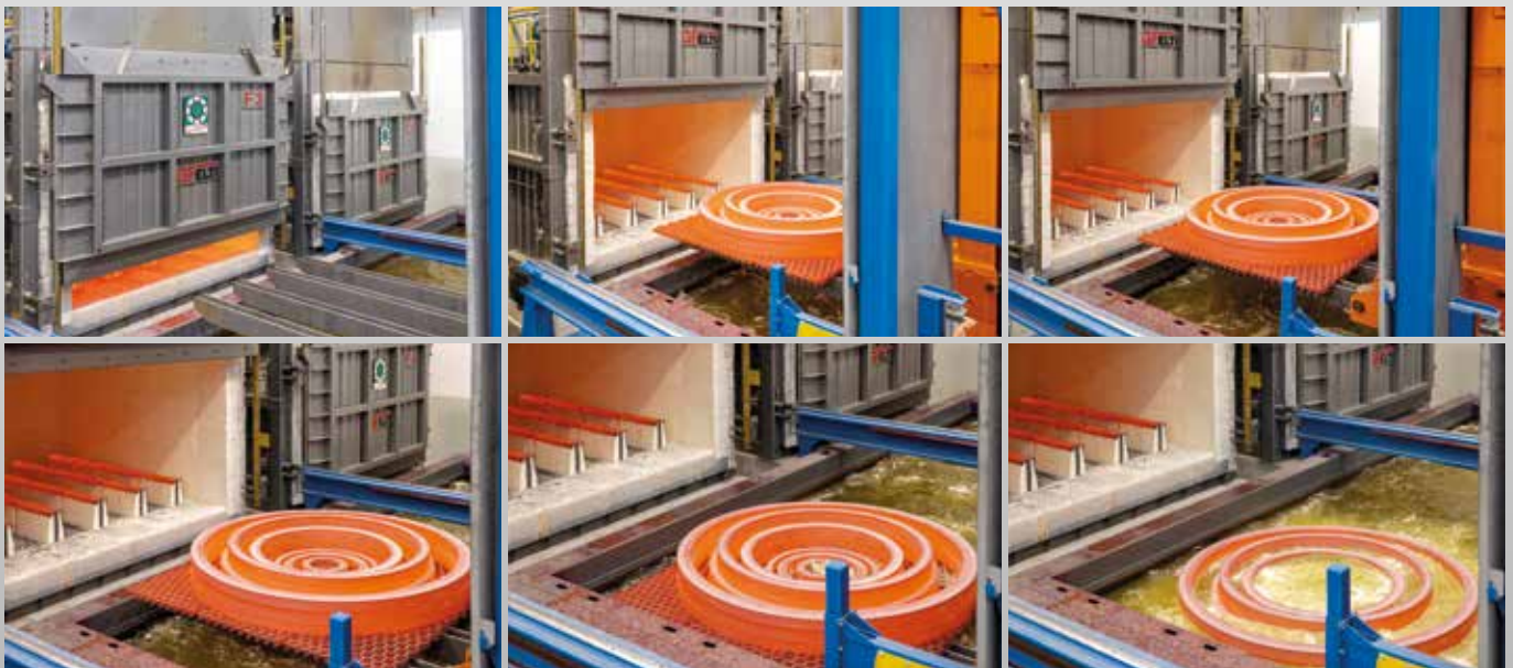
Fully automated loading and unloading heat treatment plant
